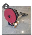
Lay the machine down with handle on the floor to fit pad/pad drive or brush.
