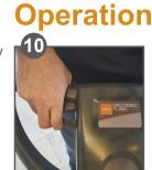
Lower handle to a comfortable position by squeezing the right lower lever.
