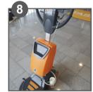
Insert water tank hose into top of machine and solution feed cord is fitted and working.
