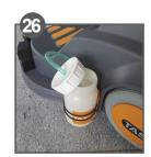
Empty spray unit and check/clean system as required (flush with clean water). Let the lid open to facilitate drying.
