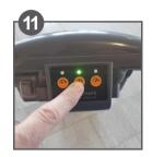
Press the correct cleaning speed button for the application.
