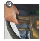
To activate machine press in orange button whilst squeezing the upper lever/s.
