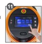
When located, choose task, check cleaning mode and number of times to carry out the task. Then press "Start".
