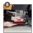
Mount brush or suitable pads for the task to be carried out.
