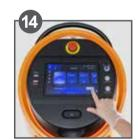
When located, choose task, check cleaning mode and No. of times carry out task. Press start.
