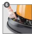
Open the front cover protection cover to access pad/brush drives.
