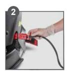
Remove machine from charger and ensure the emergency cut off switch is free (outer position).
