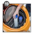
Place the filters back into position (see pictogram\* for help). Replace drainage hose when complete.
