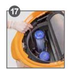
Remove plug to empty the freshwater tank. This drains through the same hose as the dirty water tank.
