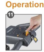
Start machine by pushing the key
