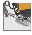
Lower brush units by using the manual lever (by foot)
