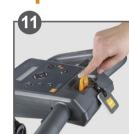
Start machine by pushing the key
