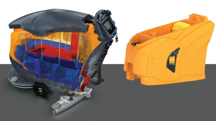
IntelliBac with antimicrobial technology is built into the tank during the tank manufacturing process. The active ingredient is added to the plastic in the rotomould.
