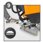
Lower brush unit by using the manual lever (by foot) or automatically by pressing the button
