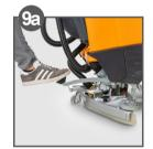
Lower brush units by using the manual lever (by foot)
