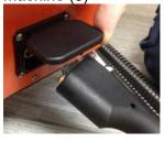
Ensuring it is pushed in all the way and the pin on the flap locks into the hole on the hose.
