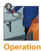
Fill solution tank with clean water.
