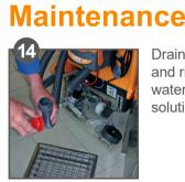
Drain recovery tank and rinse with fresh water, then drain solution tank.
