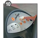
Adjust solution flow. (depending on model - with buttons on dashboard or with lever).
