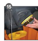
Remove the floating unit (filter and floater) with a rotation of the yellow filter in anticlockwise direction.
