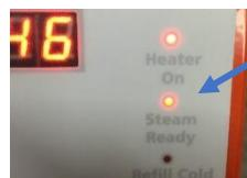
*Re-allow the temperature to increase and the steam ready light will re illuminate (9)*
