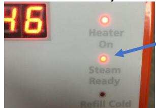
The handle controls on the steam hose are now active. The black rocker switch on the hose handle will release steam when pressed.
