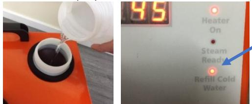
*A buzzer will sound and the steam will no longer come out of the nozzle when the steam switch on the handle is pressed.*
