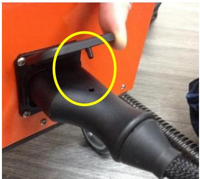
*Ensure the steam hose cannot be pulled out.*
