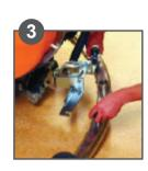
Assemble the squeegee and attach the suction hoses on both sides.
