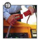
Disconnect battery and machine, connect battery and charger.
