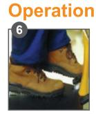
Release the foot-operated parking brake.
